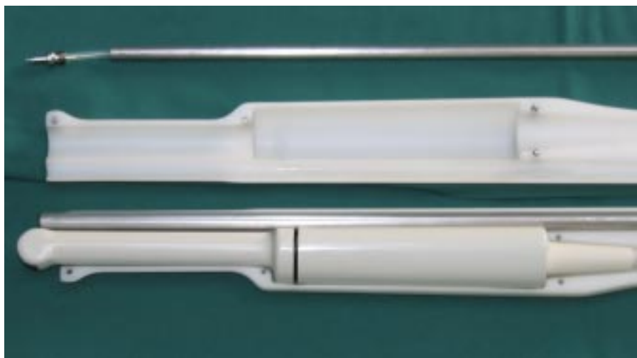
Figure 3. The R10 convex array transducer (Esaote/Pie Medical, Maastricht, the Netherlands) in a custom designed OPU probe holder (Nutricell, Campinas, Brazil)
