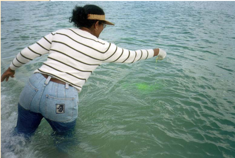
Measuring longshore currents with fluorescent dye.
