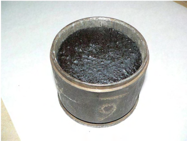
Photograph 13: Slurry before compaction
