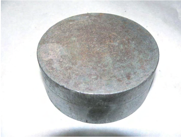
Photograph 9: Spacer block for mechanical compaction
