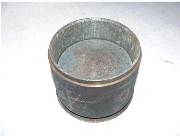
Photograph 10: Spacer block in mould
