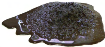
Photograph 24: Too low filler content
