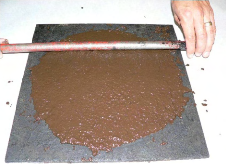
Photograph 18: Spread the slurry mix evenly
