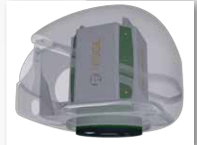
RIEGL VQ-880-G installed in the nose pod of fixed-wing aircraft DIAMOND DA42 MPP
