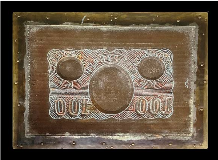
Fig. 9 Mould used by Leon Warnerke for producing forged 100-rouble notes during the 1890s. In this mould the watermark has been produced by building up layers of enamel paint and carving it down, rather than using wire. Courtesy of Peter Bower.
