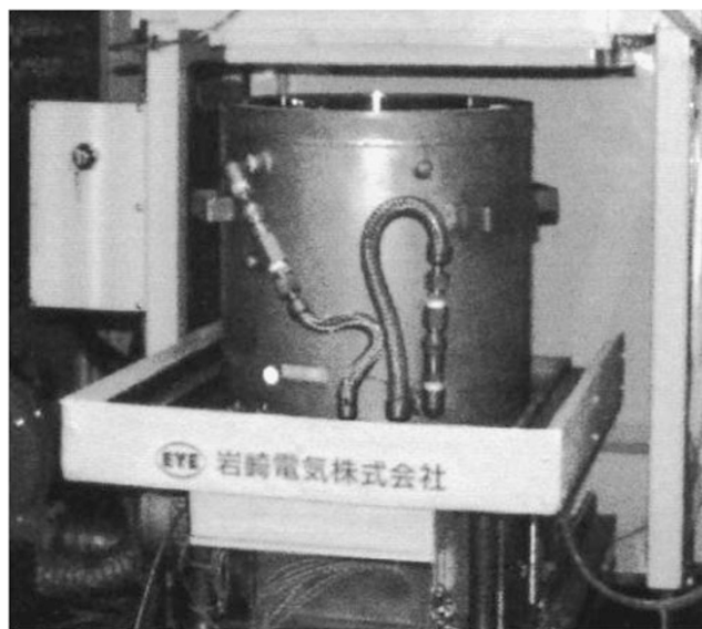
Figure 2. Reaction vessel of low energy electron accelerator (EB).
