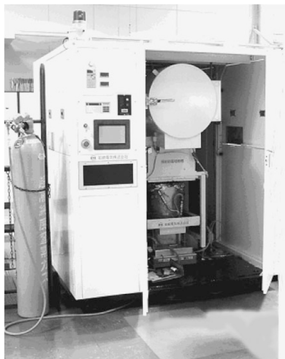
Figure 1. Front view of low energy electron accelerator pilot plant for RVNRL.
