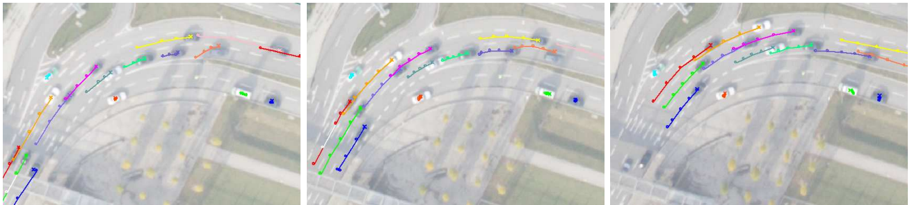
Figure 5. Test sequence with 2 fps showing frames 3, 6 and 10 in full resolution. The current vehicle position together with the recent trajectory is shown. Extrapolated trajectories are displayed in white.
