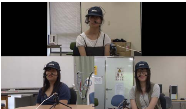
Fig. 1: Experimental setup for data collection. The caps in the participants' head are the integrated microphone and eye-tracker devices.
