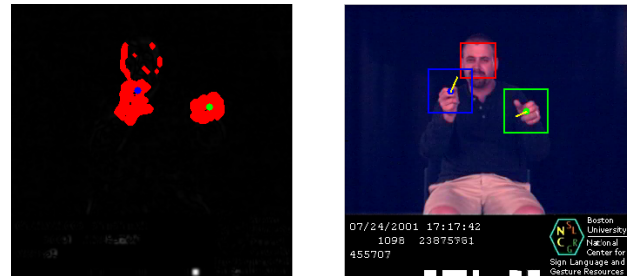
Figure 2: (a) Clustering of moving points; (b) Detected hands and face. Also displayed (in yellow) are the motion directions of the hands between successive frames.
