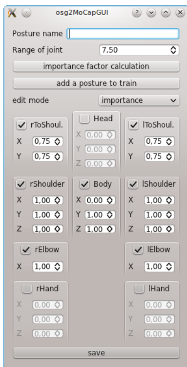
Figure 8 posture add dialog to train postures and to affect the importance (angle or range) of the joints depending on the posture
