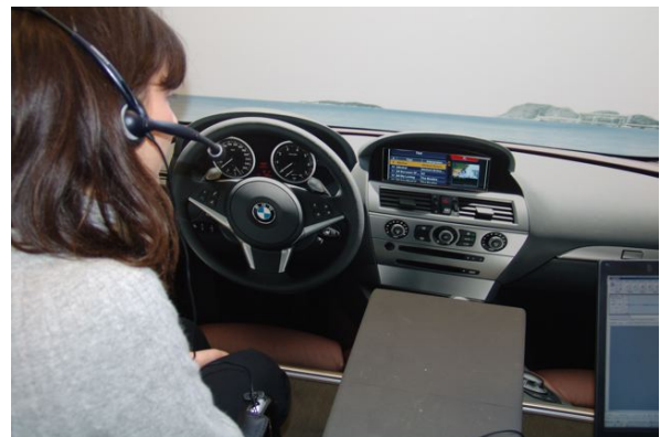
Figure 3: Experimental Setup. The subject in the mock-up system’s driver seat, investigator recording utterances and explaining tasks from passenger seat.
