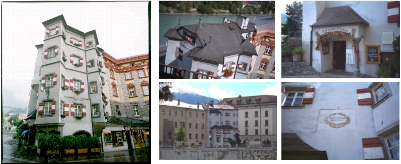
Figure 7. Examples of different images, different cameras, different lenses (from project Ottoburg, Innsbruck) to combine within a bundle solution (Hanke & Ebrahim, 1999)
