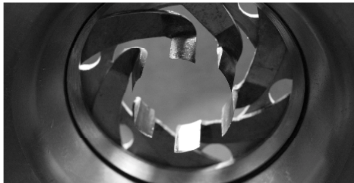
Fig. 76. The cutting head equipped with six knives
