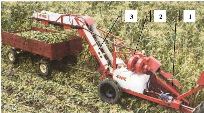
Fig. 57. Tractor-towed FMC Single-Row cob picker during work: 1– single-row cob harvesting unit, 2 – cleaning unit, 3 – belt-slat conveyor [171]
