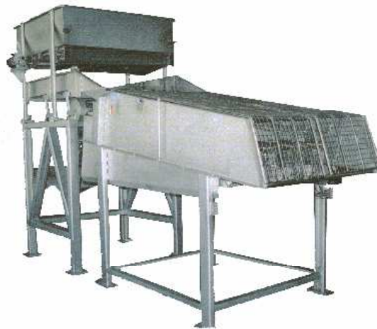
Fig. 67. The OLK-8 husker for corncob cover leaves removal [171]
