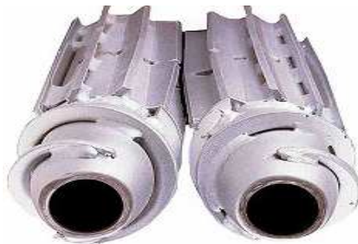
Fig. 59. Set of knives rollers for corncobs cutting [95]
