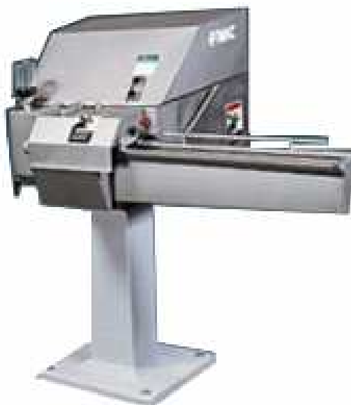
Fig. 74. The cutter of corn kernels of FMC S.C. – 120 [171]
