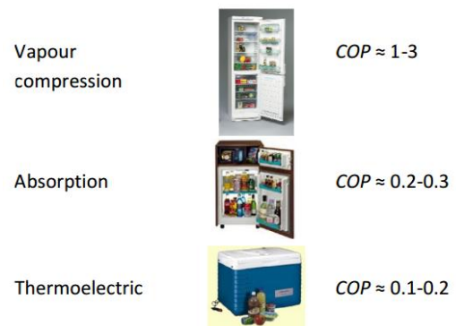
Figure 1 Different cooling principles and their typical efficiencies (ASHRAE handbook, 2010 and Granryd et al., 1999). COP (Coefficient of Performance) is a quality number defined as the ratio between the useful cooling energy and the supplied work.
