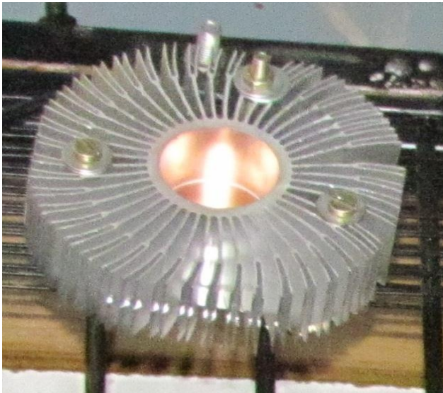
Fig 3: Heat sink install on condenser.
