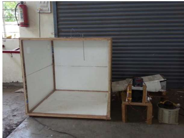
Fig. 5 Thermoelectric cooling in a 1m 3 wooden box
