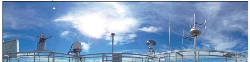
▲ Spectral sky scanner at daylight measuring site at the Technische Universität Berlin. (Source: IEA SHC/EBC Task 61 Report, Spectral Sky Models for Advanced Daylight Solutions)
