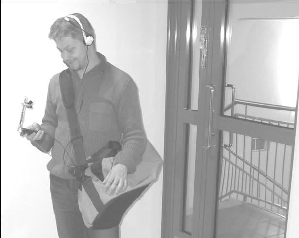
Figure 2. The test equipment: mobile phone with a miniature video camera facing the user, laptop computer in bag, headphones.
