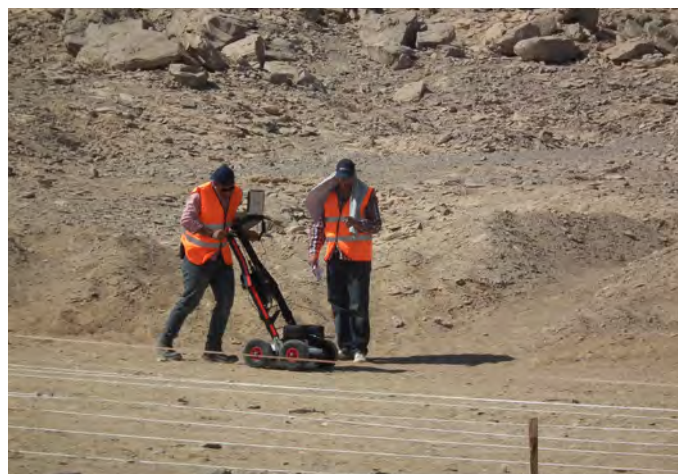
It's like mowing the road: The GPR survey underway at HK6.
