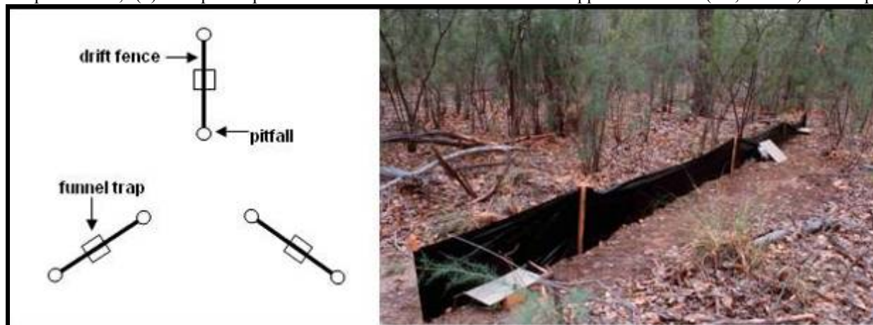
FIGURE 1. Trapping array in the riparian forest of the Middle Rio Grande, New Mexico, USA. Diagram illustrates one array with three 6-m long drift fences, oriented at 0, 120, and 240°. Six pitfalls (5-gallon buckets) with cover boards and six funnel traps were set along fences. Photograph shows one ‘arm’ of an array. (Photographed by Alice Chung-MacCoubrey).
