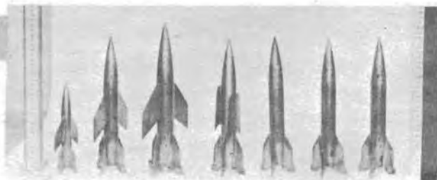
Figure 7 — Rocket Models for Supersonic Wind-Tunnel Tests
