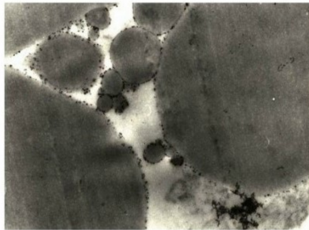
Figure 3. Microstructure of O/W emulsion containing skim milk powder (4 percent) and locust bean gum (LBG, 0.35 percent), sunflower oil (30 percent), NaCl (1.5 percent), sucrose (2.5 percent) and acetic acid (0.45 percent). Multilayers of adsorbed material and gelled zones can be observed, as well as droplet flocculation.
