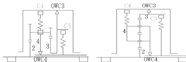
Figure 12 Automatic transmissions of three-speed changer. (Inventions 2 and 3)
