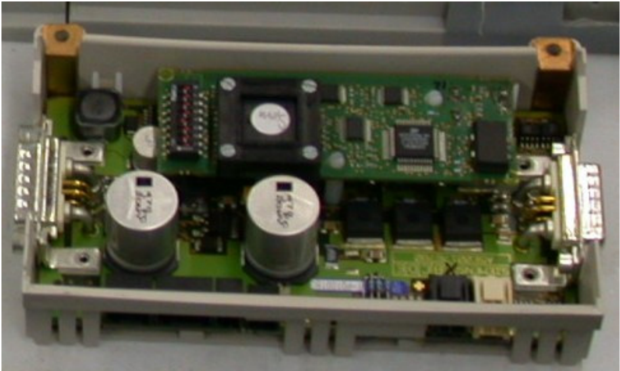
Fig.2. Realized electrical power and control unit.
