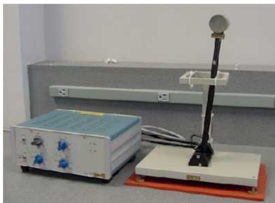
Fig. 3. IPNC plant is a GIP with an analog PID controller
