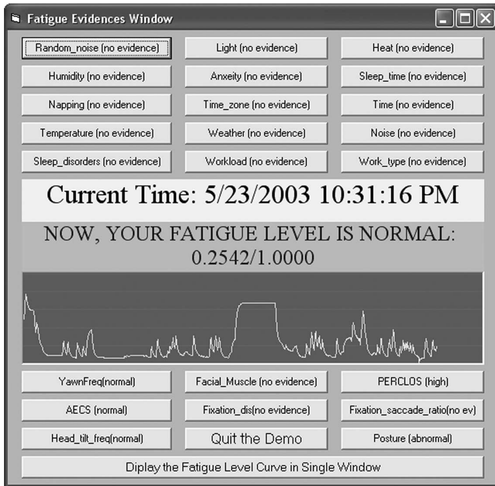
Fig. 23. Visual interface program panel, which displays the composite fatigue score over time.
