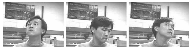
Fig. 12. Facial and facial-pose-tracking results for images randomly selected from one video sequence. The white rectangle indicates the tracked facial region and the white line represents the normal facial plane, which is drawn according to the estimated facial pose.
