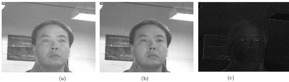
Fig. 7. (a) Even field image, (b) odd field image, and (c) the difference image.
