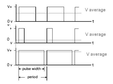
Illustration of Pulse Width Modulation (PWM)
