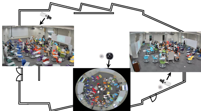
Fig. 1. The lesson video archiving system in a classroom. Two box cameras and a fish-eye camera are installed on the ceiling. The sound from the ceiling and handy microphones are also archived.
