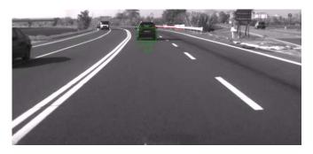
Fig. 13. Co-existence of the guard rail detection and vehicle detection algorithms: the vehicle is anyway detected also when the guard rails detection is running.
