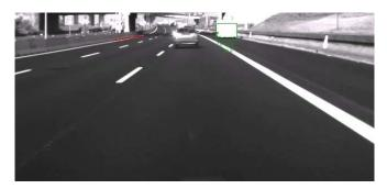
Fig. 14. Correctly detected parked vehicle. No guard rails are detected.
