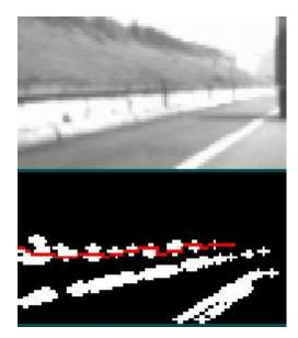
Fig. 6. Scratched guard-rail correctly detected skipping holes: red line represents found guard-rail.
