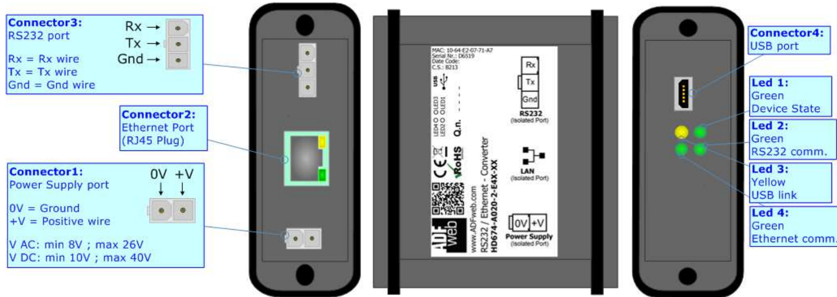
Figure 1a: Connection scheme for HD674-A020-2-E4x-xx
