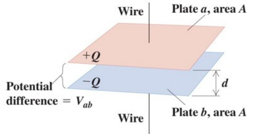
(a) A basic parallel-plate capacitor
