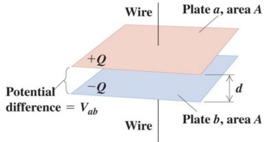
(a) A basic parallel-plate capacitor
