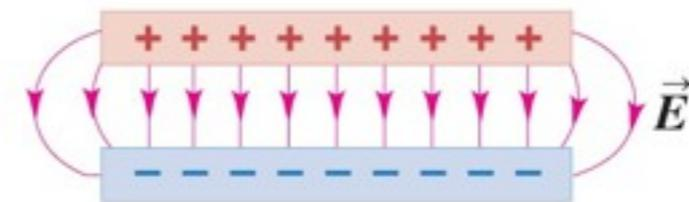
(b) Electric field due to a parallel-plate capacitor
