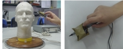
Figure 12: The 3D styling tool needs two sensors: one sensor is attached to a plastic head model, and the other one is used for controlling the editing tool.
