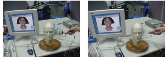
Figure 13: Clicking the buttons on the sensor can enable the scissors operation and cut selected hair.
