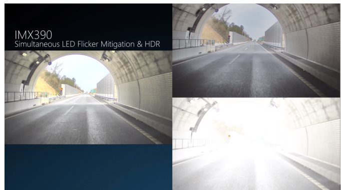
Fig. 1. IMX390 sensor sample image on a tunnel exit. The image on the left was taken with both LED flickering mitigation and High-Dynamic-Ranging (HDR) capability enabled. The top right image shows HDR functionality without LED flickering mitigation – note that the traffic sign velocity indicator does not appear. The bottom right image shows the image without any of the functionalities enabled, clearly showing the sensor capabilities. Image obtained from the Sony website [21].
