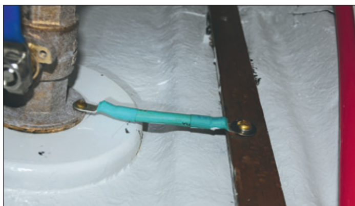
Left —Not all shaft brushes are created equal. Much like the brush contacting an electric motor's commutator, the business end that rides on the shaft should be made of carbon rather than simply a hunk of bronze pipe or rubrail. Right —A central bonding strip or bus running the length of a boat allows for bonding wires to be attached anywhere, which keeps those wire runs shorter and reduces resistance. If the strip runs along the inside of the hull well above the bilge, corrosion at connections is minimal.
