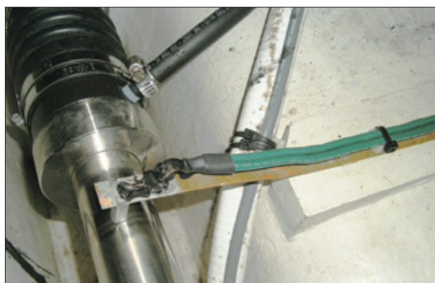
Left —Not all shaft brushes are created equal. Much like the brush contacting an electric motor's commutator, the business end that rides on the shaft should be made of carbon rather than simply a hunk of bronze pipe or rubrail. Right —A central bonding strip or bus running the length of a boat allows for bonding wires to be attached anywhere, which keeps those wire runs shorter and reduces resistance. If the strip runs along the inside of the hull well above the bilge, corrosion at connections is minimal.
