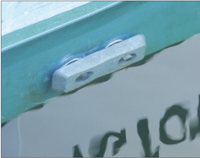
Left —When boat owners boast that their anodes last a very long time, suggest an analysis of the anodes, their attachment to the bonding system, or of the entire bonding system. Right —This corroded hull anode reveals the cast-in plate through which the mechanical and electrical connections are made to the hull. This construction ensures that consumption has no effect on the connection or security of the anode.
