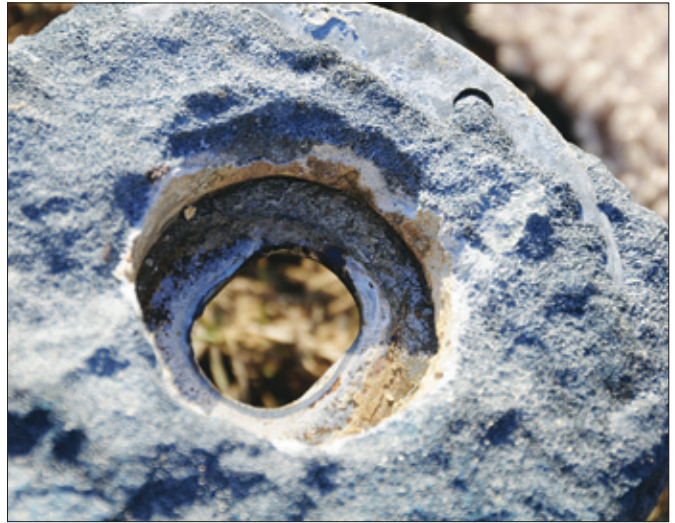
Left —When boat owners boast that their anodes last a very long time, suggest an analysis of the anodes, their attachment to the bonding system, or of the entire bonding system. Right —This corroded hull anode reveals the cast-in plate through which the mechanical and electrical connections are made to the hull. This construction ensures that consumption has no effect on the connection or security of the anode.
