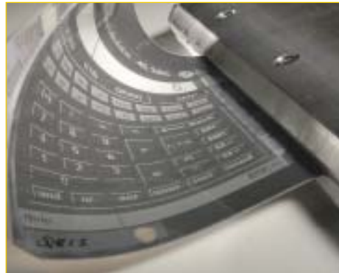
Flexible, active-matrix display produced by Polymer Vision, a venture in the Philips Technology Incubator, using Philips' ultrathin backplane and organic TFTs with E Ink's electronic ink frontplane. (Courtesy of Polymer Vision, Philips Technology Incubator.)
