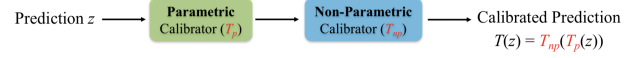
Figure 4. Composition-based calibration for achieving both high data-efficiency as well as high expressivity. The uncalibrated prediction is transformed by the parametric (or efficient) calibrator, followed by the non-parametric (or expressive) calibrator. Trainable parameters are highlighted in red.
