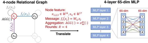
Figure 2: Example of translating a 4-node relational graph to a 4-layer 65-dim MLP. We highlight the message exchange for node x_1 . Using different definitions of x_i , f_i(\cdot) , \text{AGG}(\cdot) and R (those defined in Table 1), relational graphs can be translated to diverse neural architectures.
