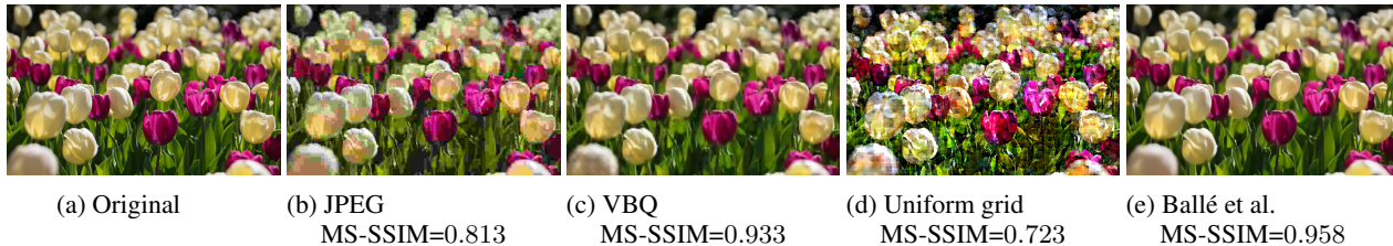
Figure 5. Image reconstructions at matching bitrate (0.24 bits per pixel). VBQ (c; proposed) outperforms AC with uniform quantization (d) and JPEG (b) and is comparable to the approach by (Ballé et al., 2017) (e) despite using a model that is not optimized for this specific bitrate. Uniform quantization here used a modified version of the VAE in Figure 6, using an additional conv layer with smaller dimensions to reduce the bitrate down to 0.24 (this was not possible in the original model even with the largest possible grid spacing).
