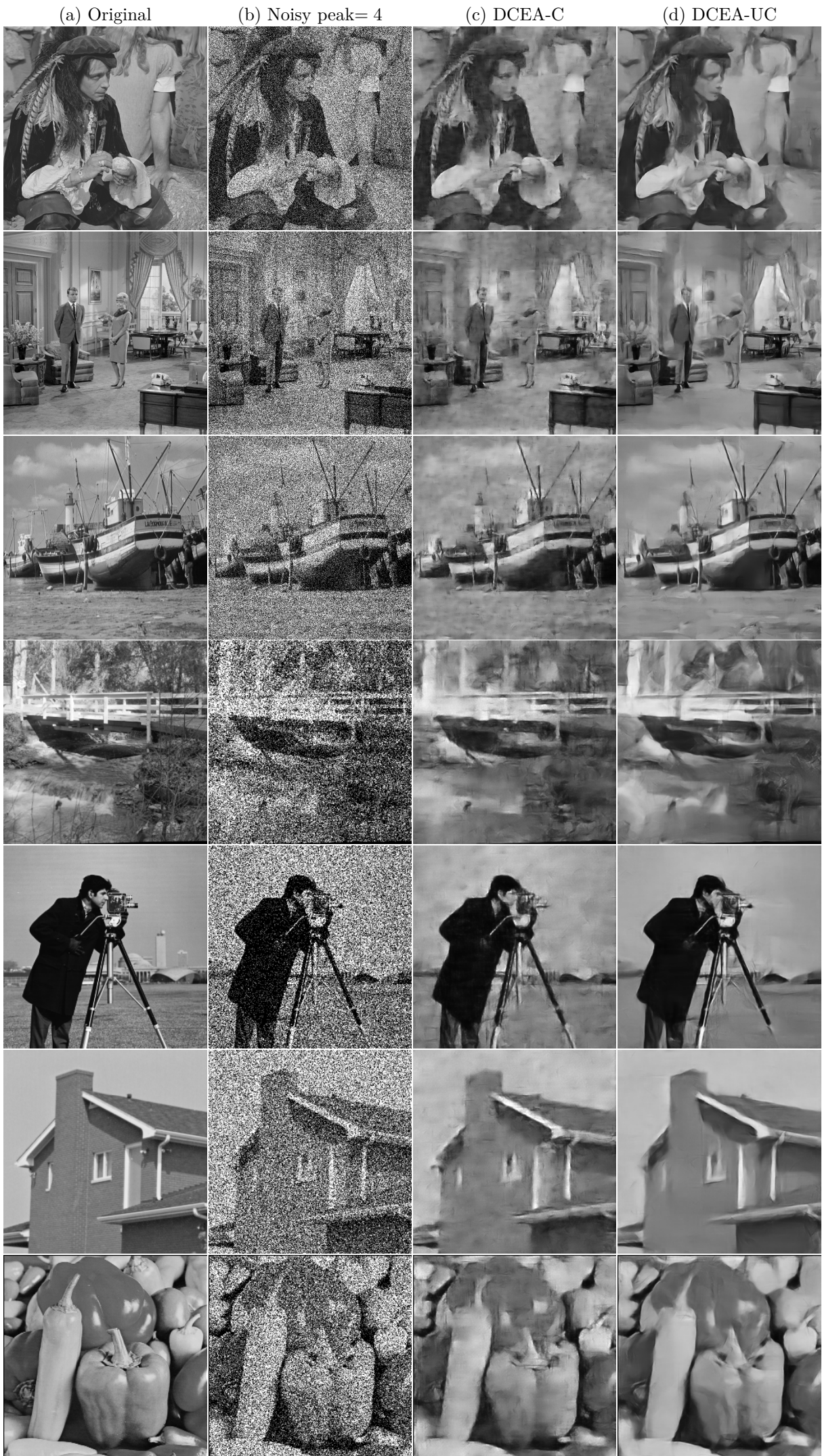
Figure 2: Denoising performance on test images with peak= 4. (a) Original, (b) noisy, (c) DCEA-C, and (d) DCEA-UC.
