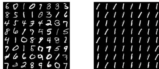
Figure 17. Images generated by a basic GAN on MNIST before and after mode collapse. The left image shows GAN-produced images early in GAN training and the right image shows GAN samples later in training after mode collapse has occurred due to training instabilities.
