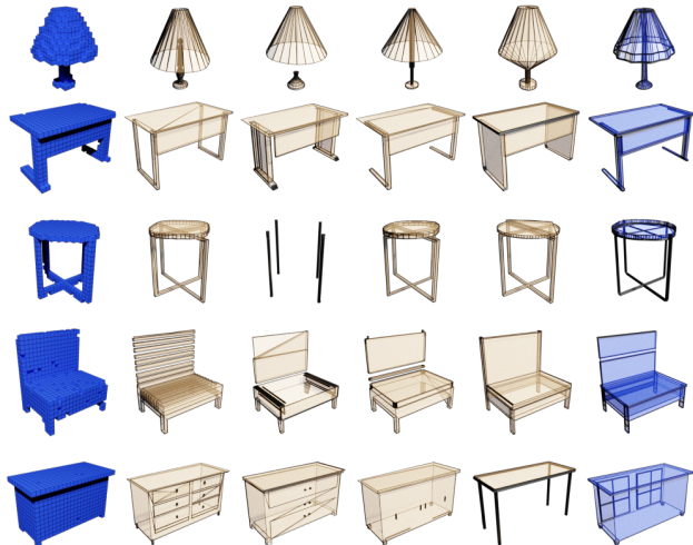
Figure 10. Voxel conditional (blue, left) samples generated using nucleus sampling with top- p=0.9 (yellow) and ground truth meshes (blue, right).
