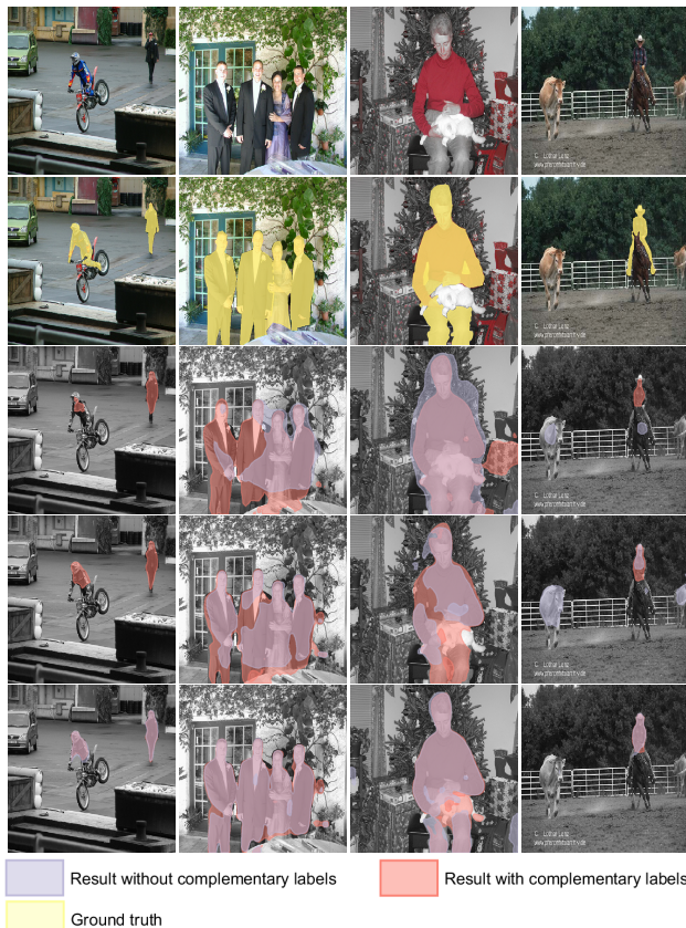
Figure 8. Segmentation results on PASCAL VOC show complementary labels improve performance in low-data settings. From top to bottom: the full image, annotations and predictions from networks trained with only the person labels ( blue ) and predictions from a network trained with both person labels and complementary labels ( red ) using N = \{200, 500, 1464\} training examples.
