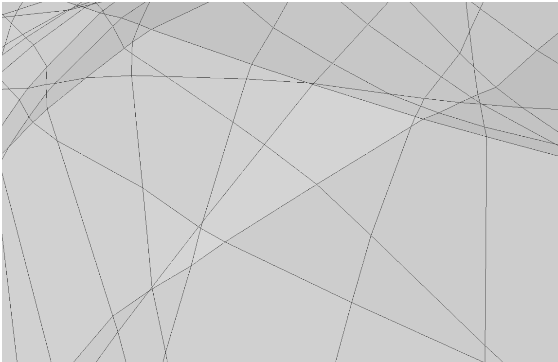
Figure 5. A local surface area of the polygonal mesh produced by analytic marching, which is obtained by further zooming in the focused area of our “Sofa” result reported in Figure 3 of the main text. Note that the polygonal mesh produced by analytic marching can be easily converted as triangle mesh, simply by connecting diagonals on individual polygonal faces.
