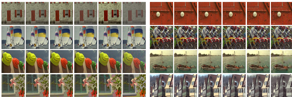
Figure 15. Examples from the TID2013 data set proposed by Ponomarenko et al.. Displayed are a change of contrast, three types of noise, denoising, jpg2000 compression, and two color quantizations (from left to right and top to bottom).
