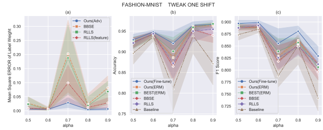
Figure 2. (a) Mean squared errors of estimated label weights (Lower is better), (b) accuracy and (c) F-1 score (Higher is better) on FASHION-MNIST for the uniform training set and Tweak-One shifted test set, where \alpha is the probability of the tweaked class.
