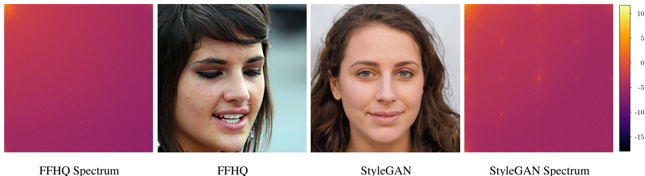
Figure 1: A side-by-side comparison of real and generated faces in image and frequency domain. The left side shows an example and the mean DCT spectrum of the FFHQ data set. The right side shows an example and the mean DCT spectrum of a data set sampled from StyleGAN trained on FFHQ. We plot the mean by averaging over 10,000 images.
