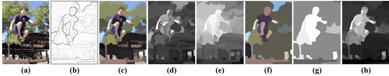
Fig. 2. Illustration of region segmentation and regional saliency measurement. (a) original image; (b) ultrametric contour map; (c) primitive region segmentation result; (d) global contrast map; (e) spatial sparsity map; (f) coarse region segmentation result; (g) object prior map; (h) initial regional saliency map.
