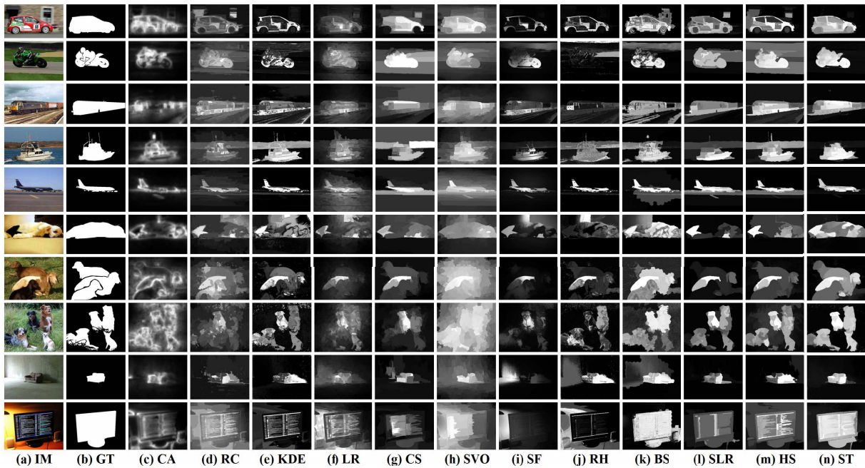
Fig. 11. Examples of saliency detection on PASCAL-1500 dataset. (a) images (IM), (b) ground truths (GT) and (c)–(n) saliency maps generated using different models.
