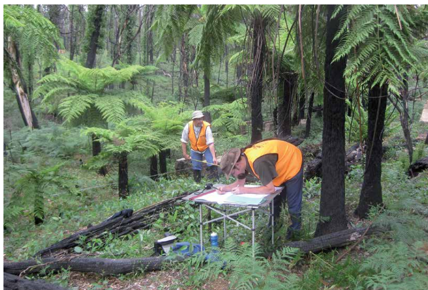
Scott Gould measuring from a datum line and Stuart Thyer plotting the position of various elements of the mill site on a gridded sheet on 17 January 2010 Photo: Mal Dow
