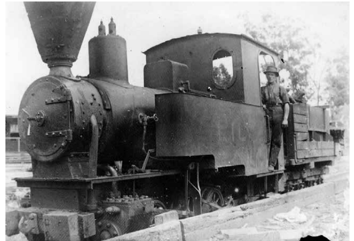
3771 on the Goodwood Tramway with substantial water tanks and a timber bogie tender B McMaster courtesy Mike McCarthy
