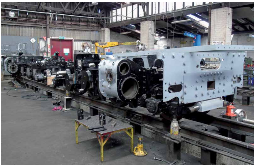
Work on NG/G16-129 continues at a steady pace, with the engine units being trial fitted to their wheels Photo: Michael Chapman, 9 October
