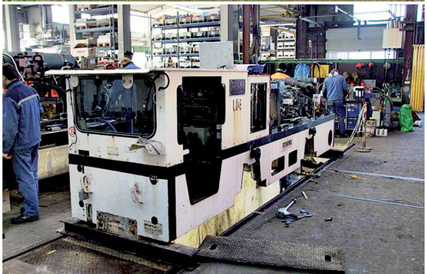
Top: On loan to Proserpine Mill from Inkerman Mill, EM Baldwin 0-6-0DH Carstairs (6/2715.1 9.68 of 1968) is seen here in the Kelsey Creek area on 14 September. Photo: Scott Jesser Above: Undergoing an extensive re-manufacture process at the maker's plant in Diepholz Germany, former John Holland Group Schöma tunneling locomotive L04 (6245 of 2008) was showing signs of the storage period when seen here on 1 February 2012. Photo: Ulrich Völz
