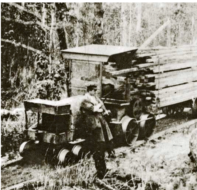
The failed 'Munro' tractor on Hayden's tramline in the Otways. (The front bogie appears to be derailed). The tractor was no more successful on Dumbrell's tramway. Photo courtesy Norm Houghton
