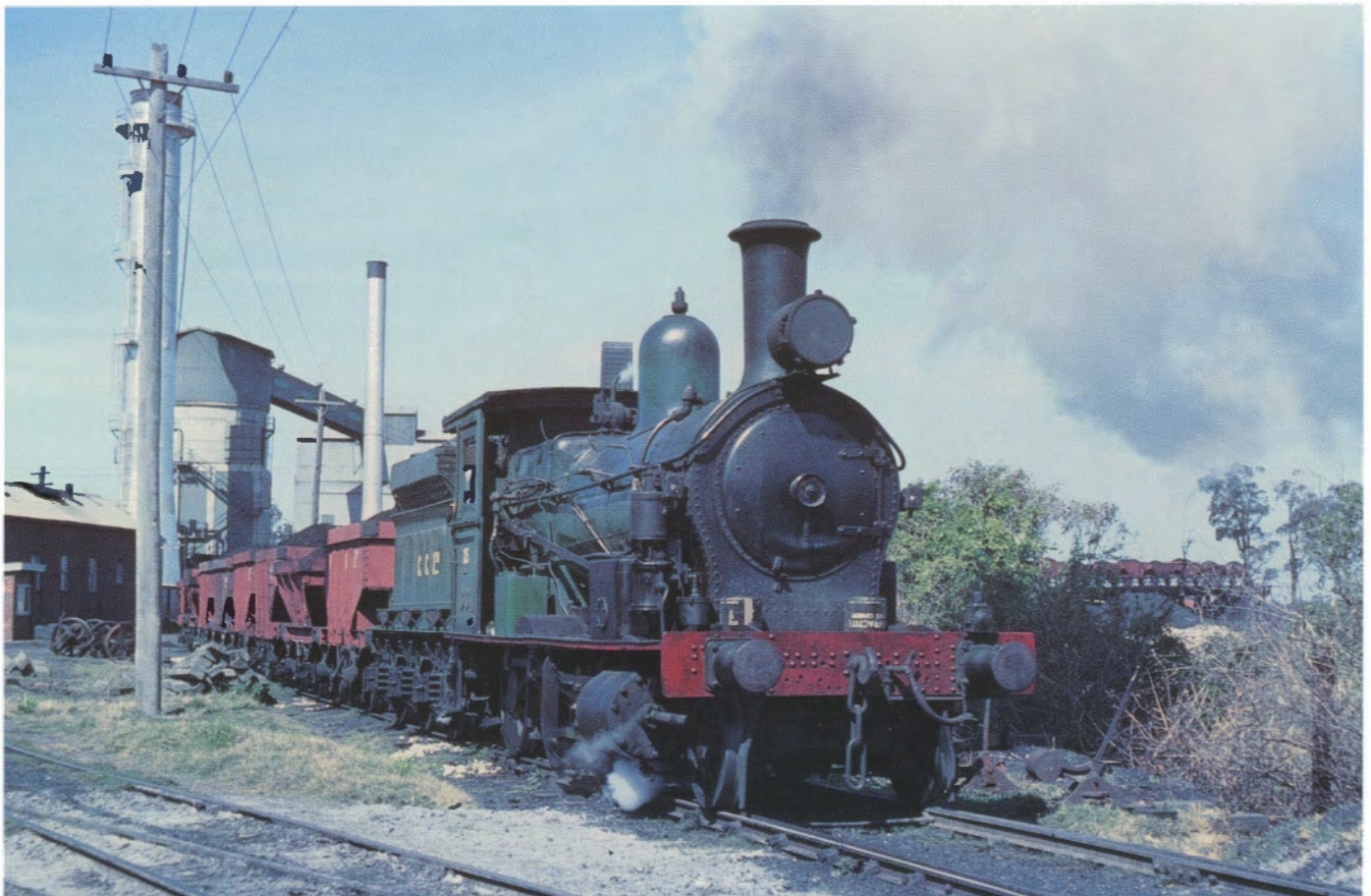
CC&C 2-6-0 number 25 (formerly NSWGR 2535, Beyer Peacock 2322 of 1884) shunting loaded hoppers in the yard at Corrimal, 28 September 1962. The loco shed is on the left, while the power house chimney rises behind. Photo: Ted Skiller, courtesy ARHS (NSW) Railway Resource Centre
