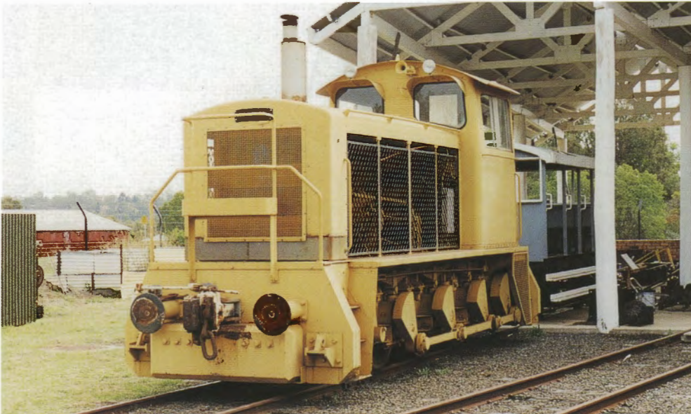
Warwick Rail Museum: ex-Mackay Harbour Board 3ft 6in gauge ComEng 0-6-0DH (F1018 of 1957) with Caterpillar engine, 10 April 2003. Photo: Brian Webber
