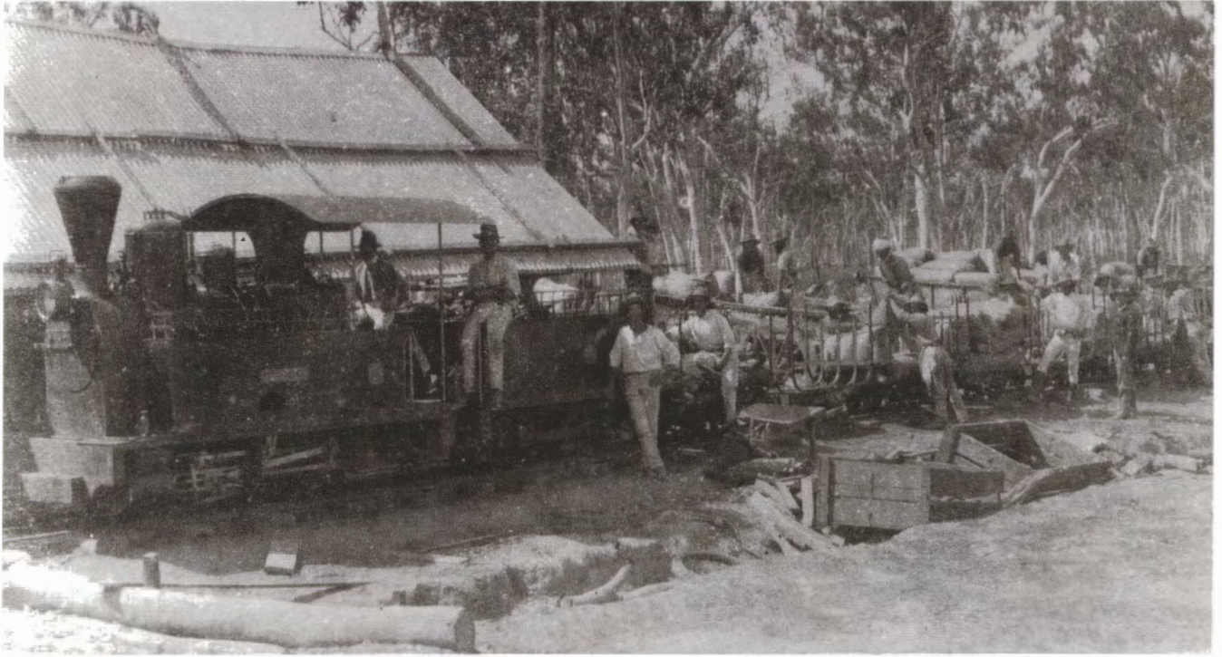
A raw sugar train at Baker's Creek, the railhead for Mackay, in 1883. PETIT BOURG is adjacent to the sugar shed and the debris of line construction is apparent. The paintwork of the Decauville tender still appears to be gleaming and the sugar has been carried on Decauville cane trucks. The locomotive's headlight is one "to kill for"! Photo: Noel Butlin Archives Centre, ANU. CSR Deposit 142/3649, p.66, Negative 6027
