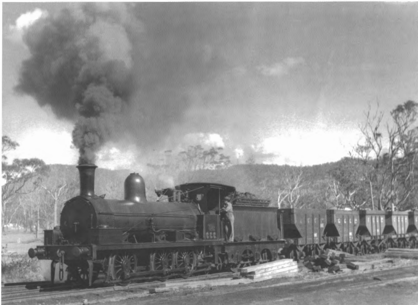
Built by Robert Stephenson and Co. in 1864, No.18 served the NSWGR as a member of the E-17 class until it was sold in 1897. The 0-6-0 moved to Corrimal in 1912 where it operated until 1964 and was withdrawn after an active life of some 78 years.. Polished and cleaned, the veteran brings another load of vertical-sided hoppers to the Corrimal coke ovens in 1955 Photo: Ron Preston
