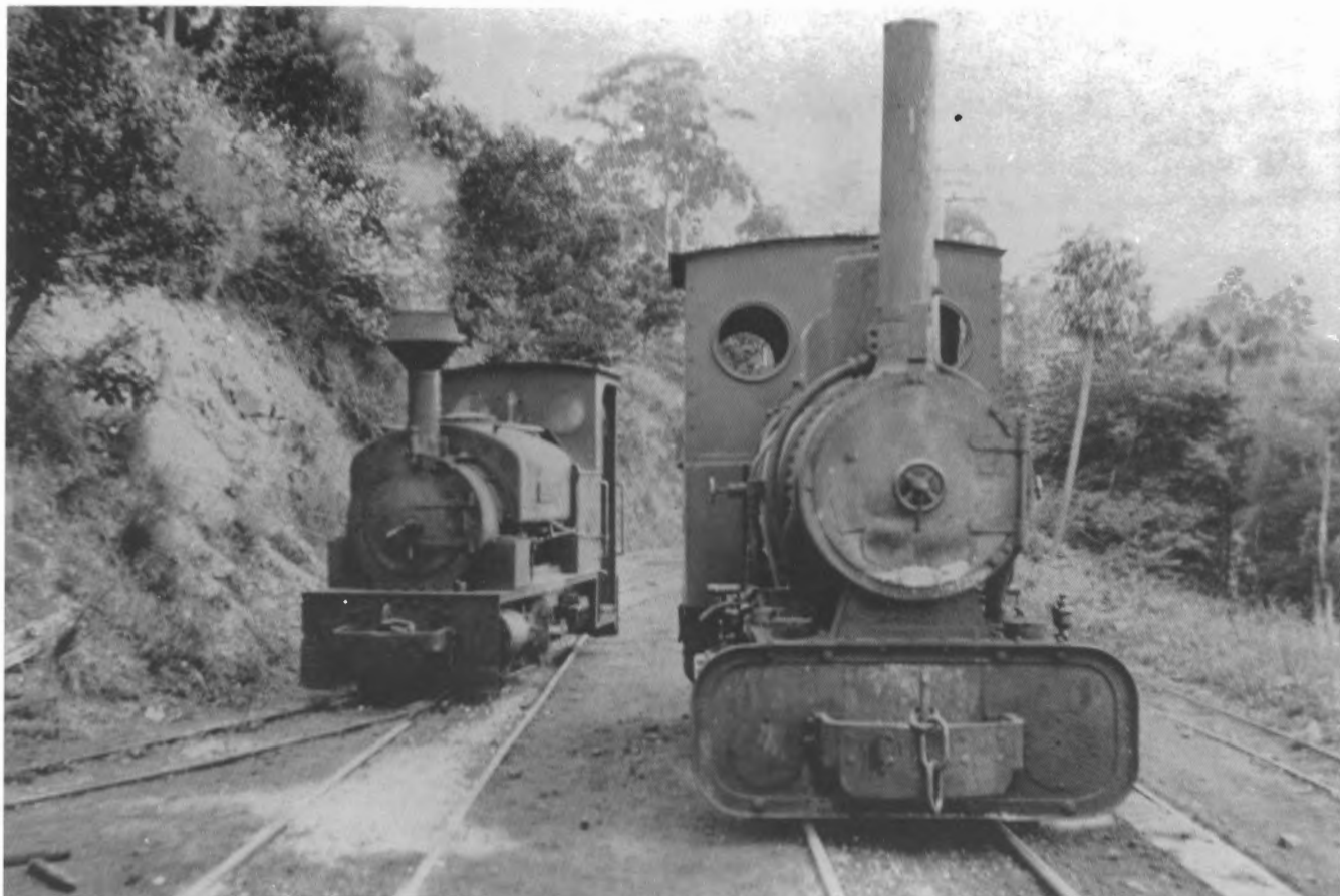
In the early 1930s when the narrow gauge was very busy, BURRA was assisted by a 10-ton 0-4-0WT Krauss (6927 of 1914), which remained in service from 1914 until 1944. At this time, BURRA was fitted with a diamond spark arrester funnel and still had its original British-style smokebox door. The pair is shown circa 1934 standing in the mine yard, adjacent to the engine shed. Photo: Author's Collection
