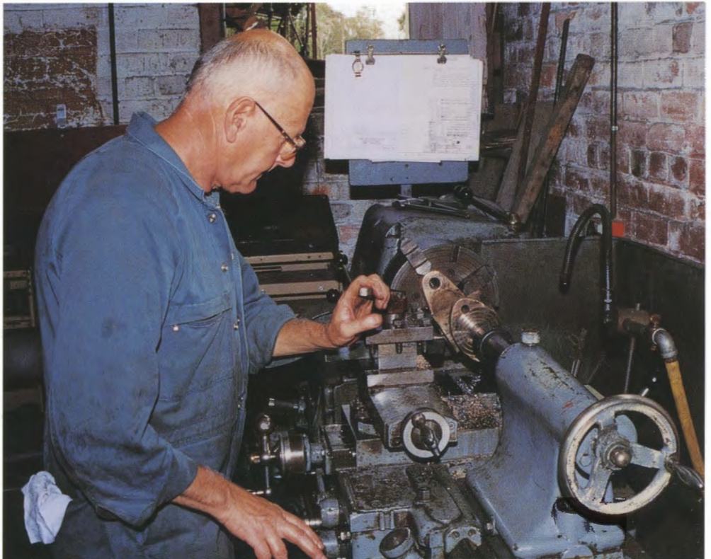
Prior to the big day, Richmond Vale Railway & Museum member Max Dixon is busy machining the blowdown valve from No.30.
