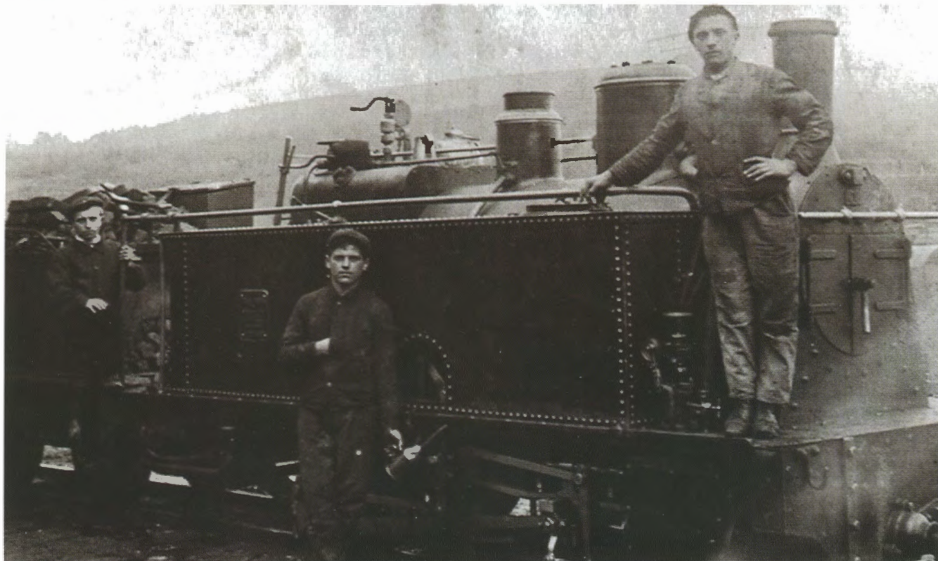
Couillet 622 of 1883 was a 700mm gauge locomotive supplied to an ironstone mine in Luxembourg and shared many similar features with the ones supplied to CSR for use in Queensland and Fiji. Photo: Emile Kreins collection courtesy Jean-Marie Otelé ( http://www.rail.lu/couillet.html )
