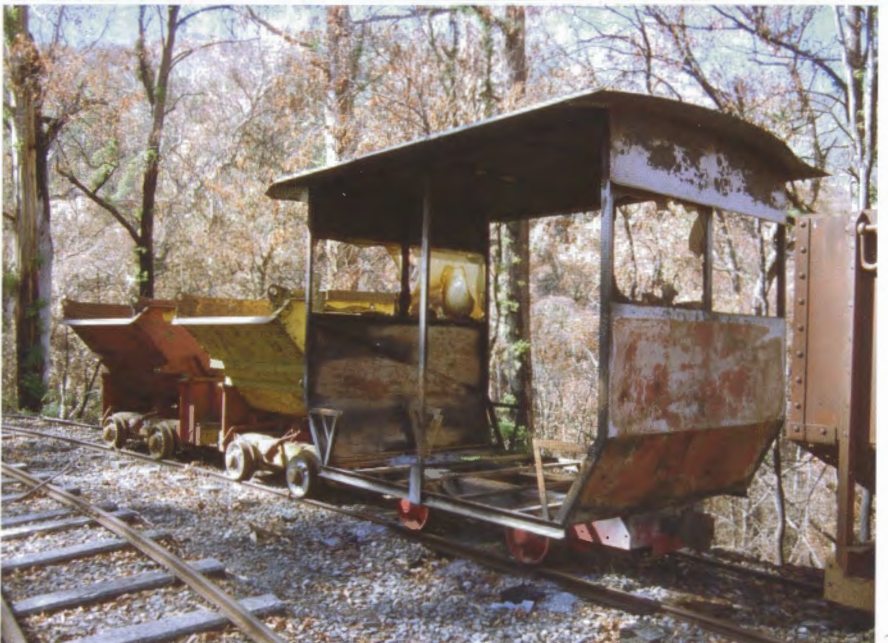
Top: The post-bushfire autumnal shades contrast with the sylvan green of the shed at the terminus of the 3ft gauge Bogong Creek tramway in Victoria. Photo: Vic Greensill Above: This passenger car, built on the chassis of a tip wagon, was burnt out in the bushfires that damaged the Bogong Creek tramway. The steel tip wagons behind fared a bit better. Photo: Colin Harvey
