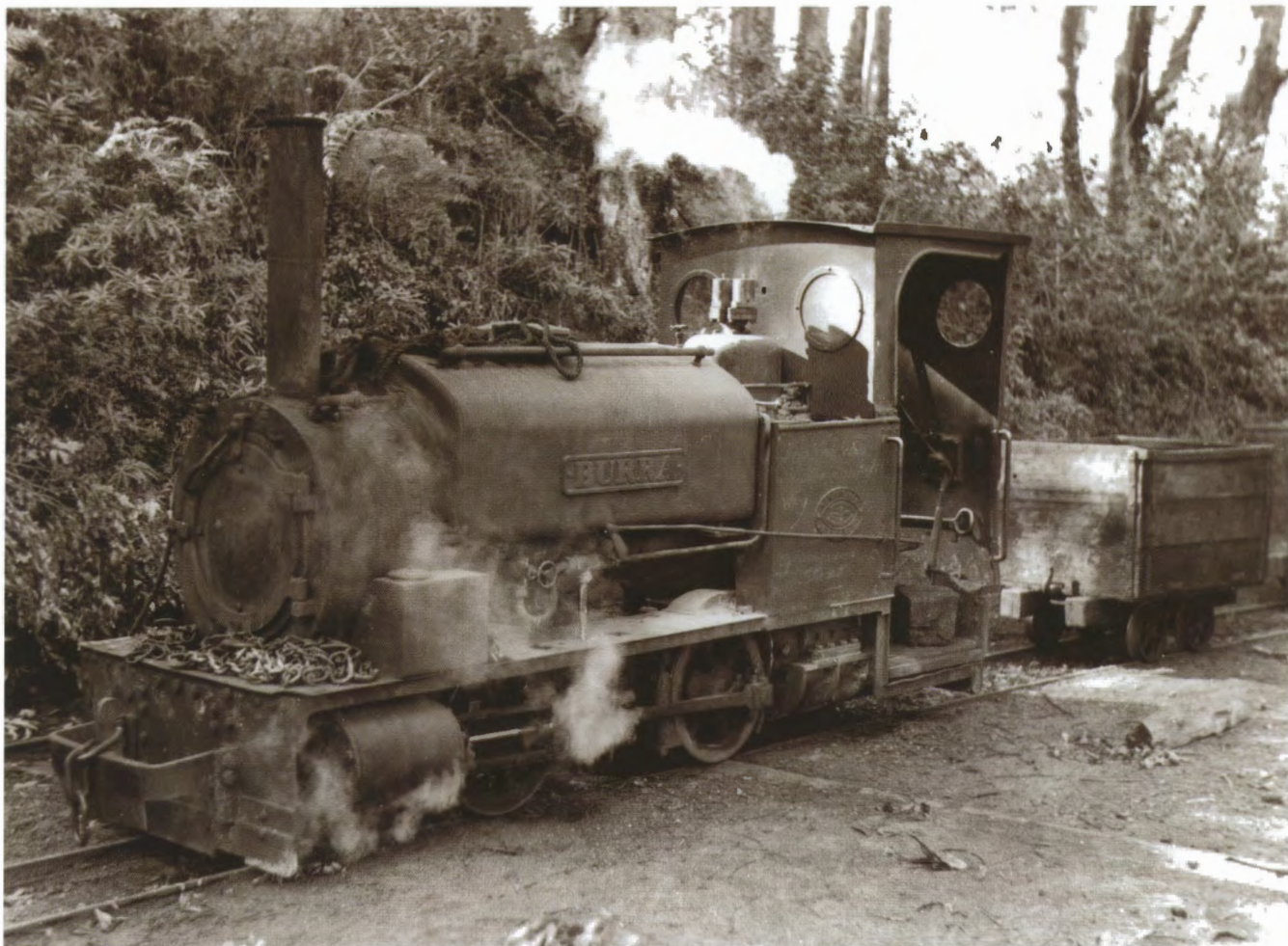
The tiny 0-4-0 saddle tank BURRA spent its entire working life on the isolated two foot gauge railway set high on the side of the escarpment above Corrimal. Built by Hawthorn Leslie & Co. Ltd in 1923, the little loco is shown fitted with the replacement boiler of 1943, built locally by Clyde Engineering, on which bureaucracy insisted that full size fittings be used.
