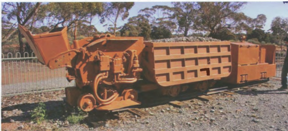
Bill Hanks photographed this display of underground mining railway items on static display at the Kambalda Tourist Information Centre in October 2008. The 762mm gauge Clayton 4wBE locomotive, Gramby car and EIMCO 12B bogger are believed to have come from the Western Mining Corporation.
