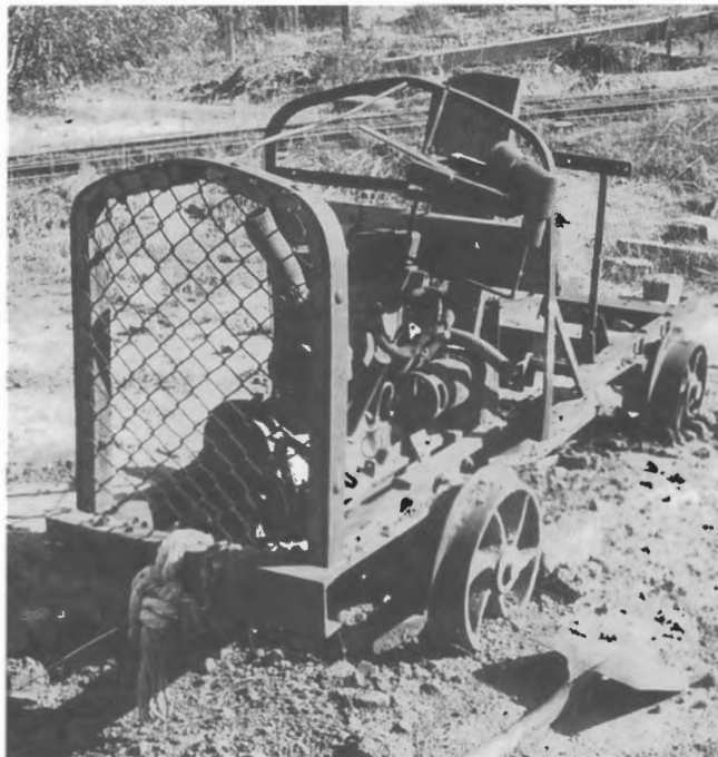
Whiteman's first locomotive was this converted Chevrolet Peacock truck. It had clearly not been used for many years when Keith McDonald photographed it at the brickworks in February 1971.
