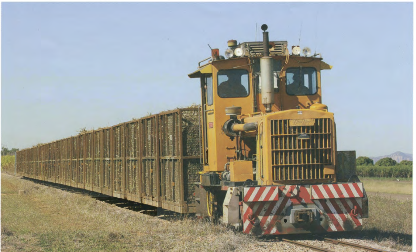
Kalamia Mill's Com-Eng 0-6-0DH CHIVERTON (C1030 of 1958) was sent to Dalbeg to operate what had become an isolated tramline of Invicta Mill as a result of the flood damage to Expedition Pass Creek bridge. Here it is handling a short rake of full bins on 7 August.
