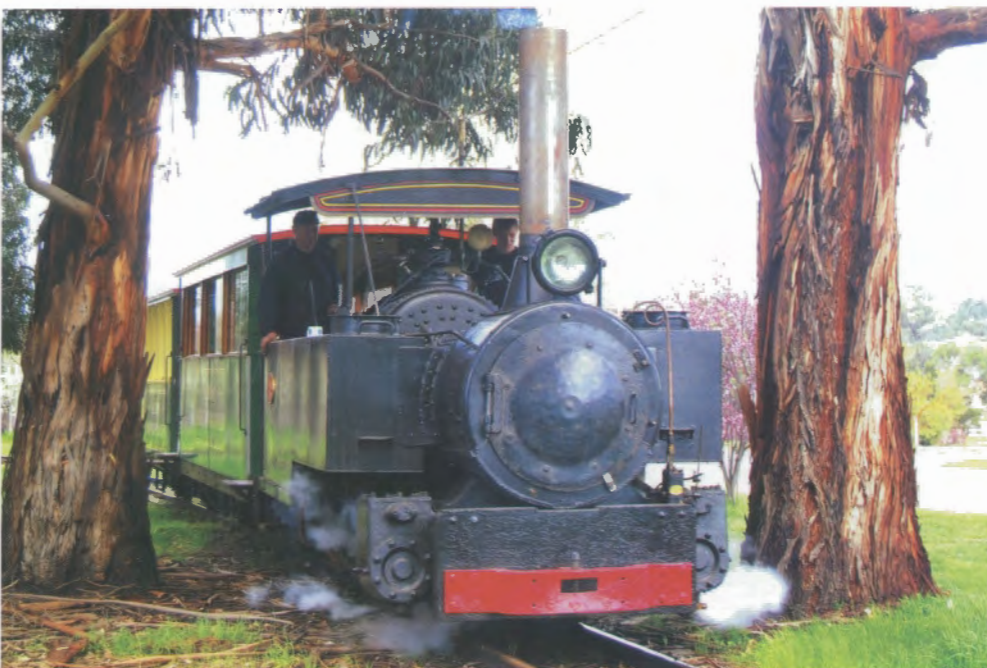
0-6-0T John Fowler 11885 of 1909 undertakes its successful in-service test run at the Alexandra Timber Tramway on Sunday 14 September 2008. Note the temporary 'stove-pipe' funnel. Photo: Peter Evans
