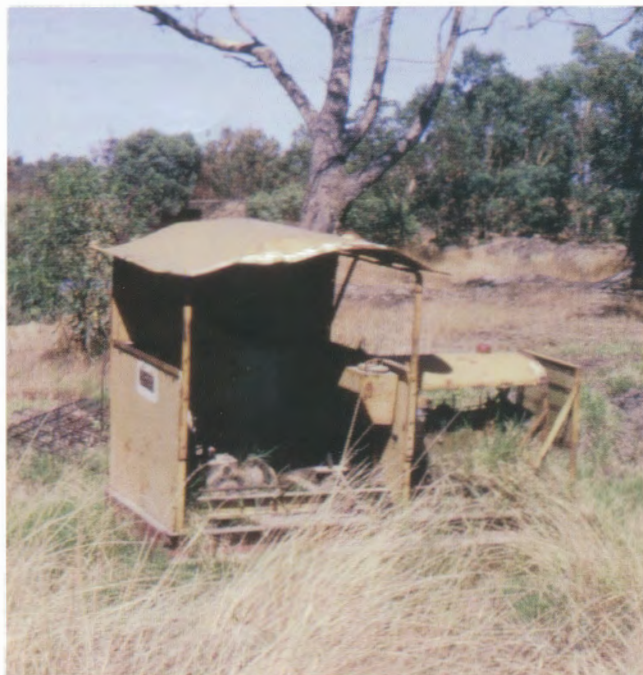
The first Planet 4wPM locomotive YELLOW ROSE (Hibberd 2055 of 1937) rusts away in the long grass near the clay pit, February 1983. Photo: Lindsay Watson
