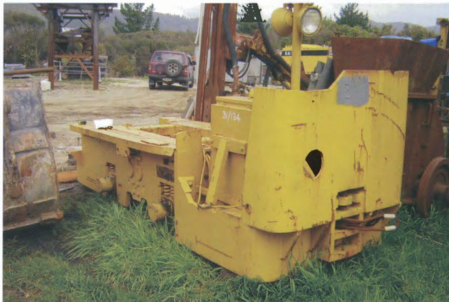
Ex Mt Isa Mines Gemco 4wBE 55 (6B/5691-6B/6101/66/68) at Charleston, on the west coast of New Zealand's South Island, 2 October 2008. The axle arrangement shows that it was built as a gauge convertible unit. Photo: Paul Napier
